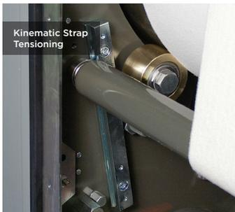
Kinematic Strap Tensioning
